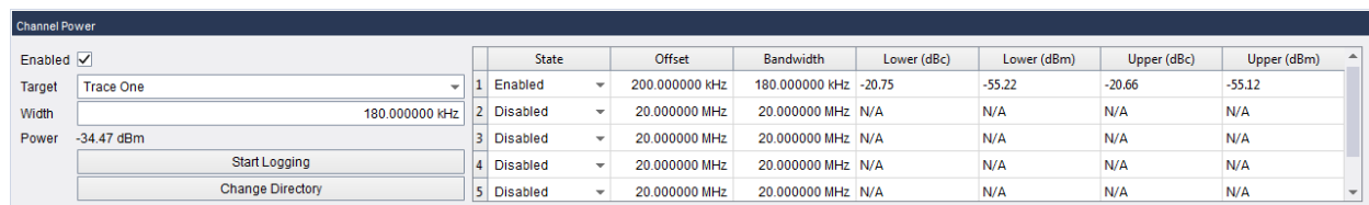
Figure 48: Channel Power control panel measuring a broadcast FM signal.
