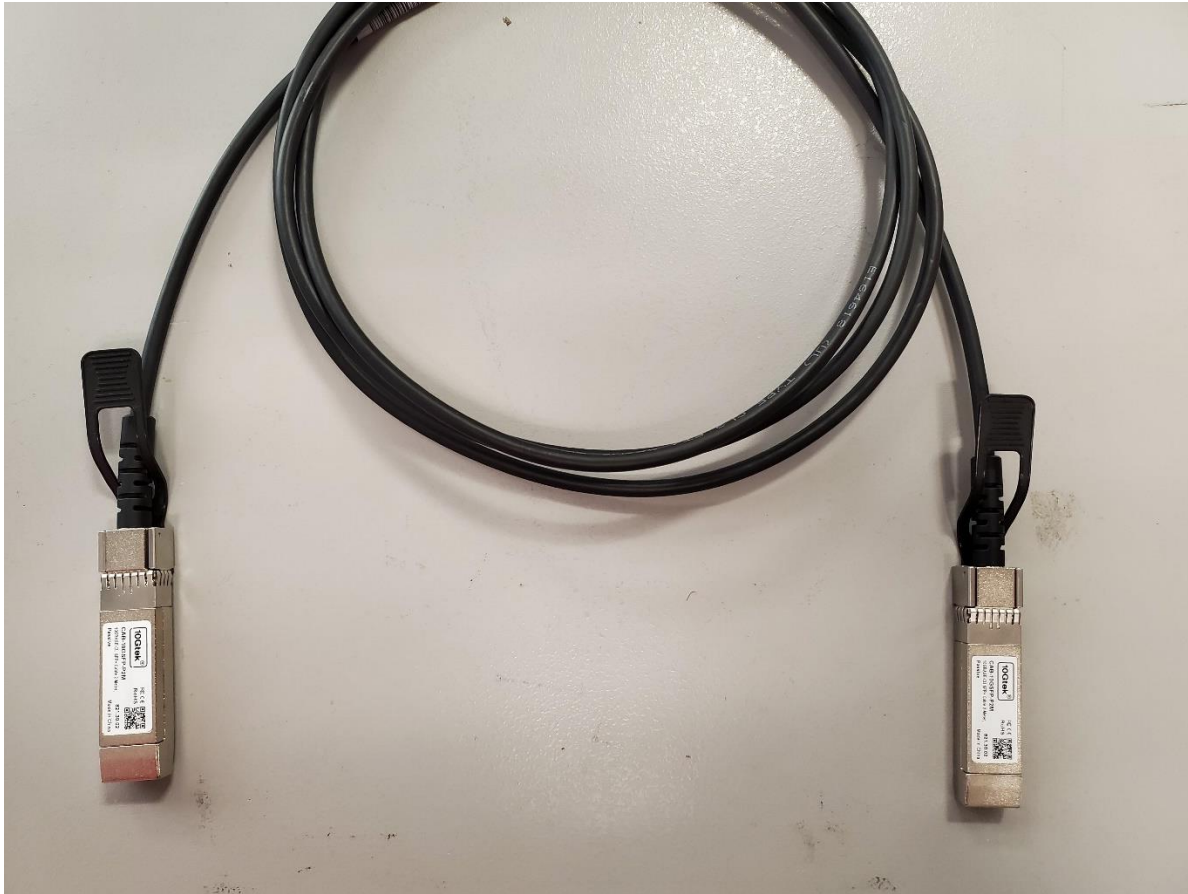
Figure 2: 10GbE copper cable. Terminated with two non detachable SFP+ modules.
