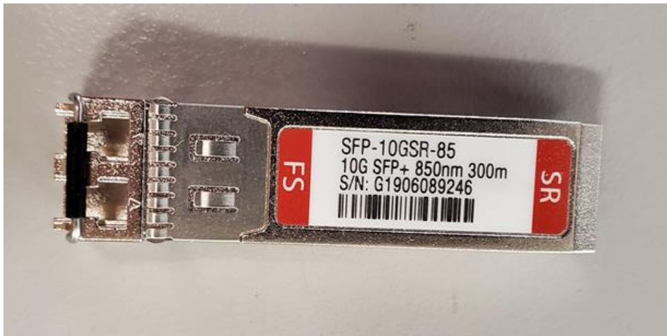
Figure 1: SFP+ 10GBASE-SR (fiber optic) module
