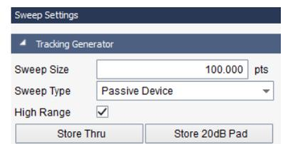
and lower range readings. This is only used for settings of High Range, Passive Device. If you omit this step, accuracy below -40 dB should be treated as +/- 1 dB typical.
