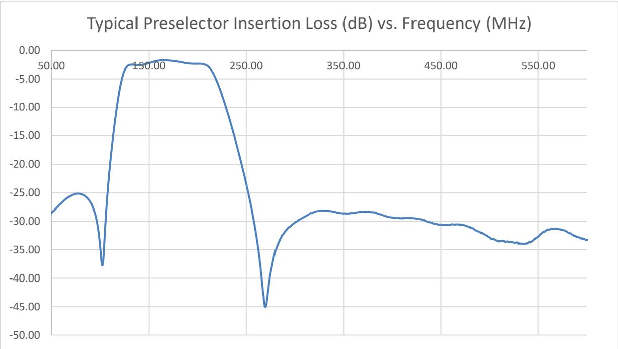
When using optional preselector filters with I/Q streaming, or when predicting if a preselector will help block an interfering signal, use the tables below.
