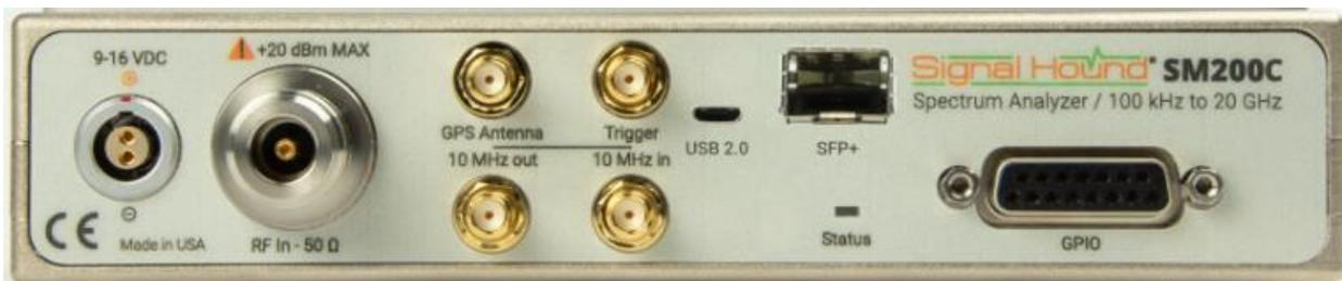
1. 9-16V DC power input: Use the included 12V supply, or a battery that can source 40 watts.
