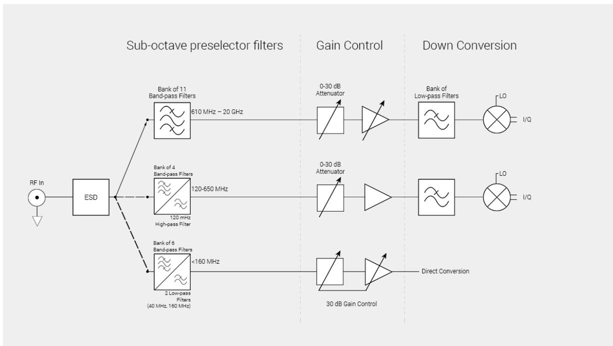
The SM200 is essentially a low IF receiver. We chose this architecture to complement our low phase noise local oscillator (LO), while avoiding the shortfalls of zero IF (direct) conversion, and because of the availability of high linearity direct conversion demodulators and I/Q mixers.
