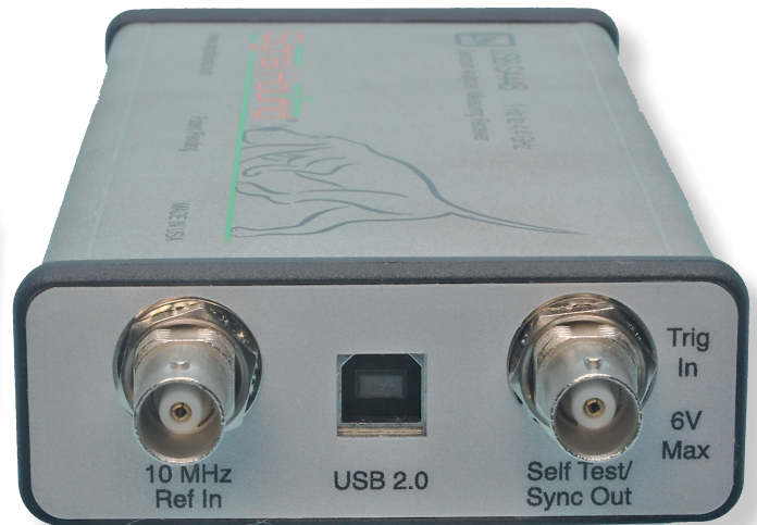
Front (above) and rear (right) panels of the Signal Hound USB-SA44B, just a bit larger than life size. There are no controls as such – they’re all taken care of via the supplied software.
