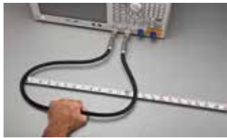
Flex Test (one full cycle)
